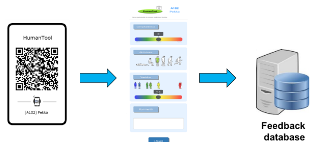
Fig. 7. QR code technology for giving personal feedback of experienced Indoor Environment Quality.
